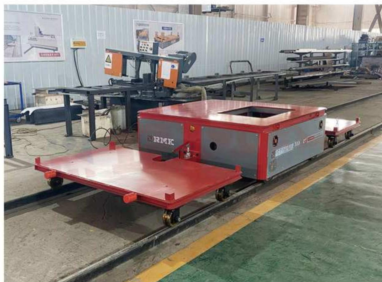
运载+牵引两用RGV——钢铁 & 冶金 Dual use RGV for transportation and traction - Steel & Foundry
