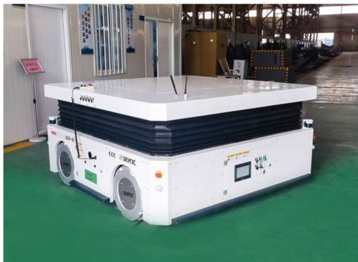
激光+磁条+二维码混合导航麦克纳姆轮式AGV——航天军工 Laser + magnetic stripe + QR code hybrid navigation McNAM wheel AGV - Aerospace & Military
