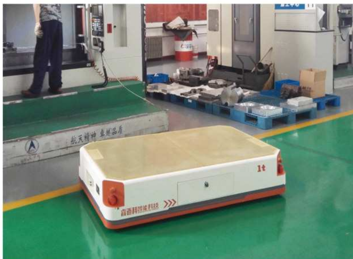
1吨无轨电动平车——航天军工 1 ton trackless transfer cart - Aerospace & Military
