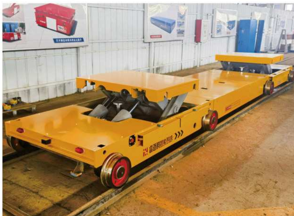
35吨升降RGV——军工 35 tons lifting RGV - Military
