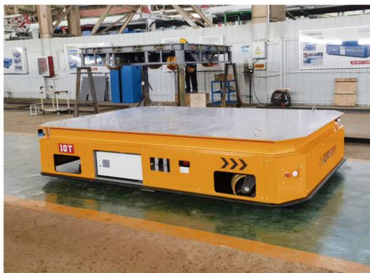
10吨全向移动车——航天军工 10 ton omnidirectional mobile transfer cart - Aerospace & Military
