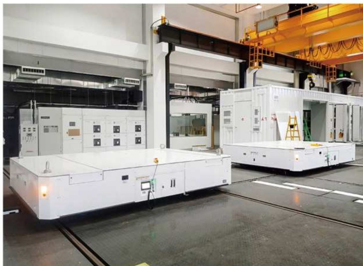
40+40吨双车联动纵横移动RGV——储能 40+40 Ton Double-Vehicle Coordinated Vertical and Horizontal Moving RGV - Power
