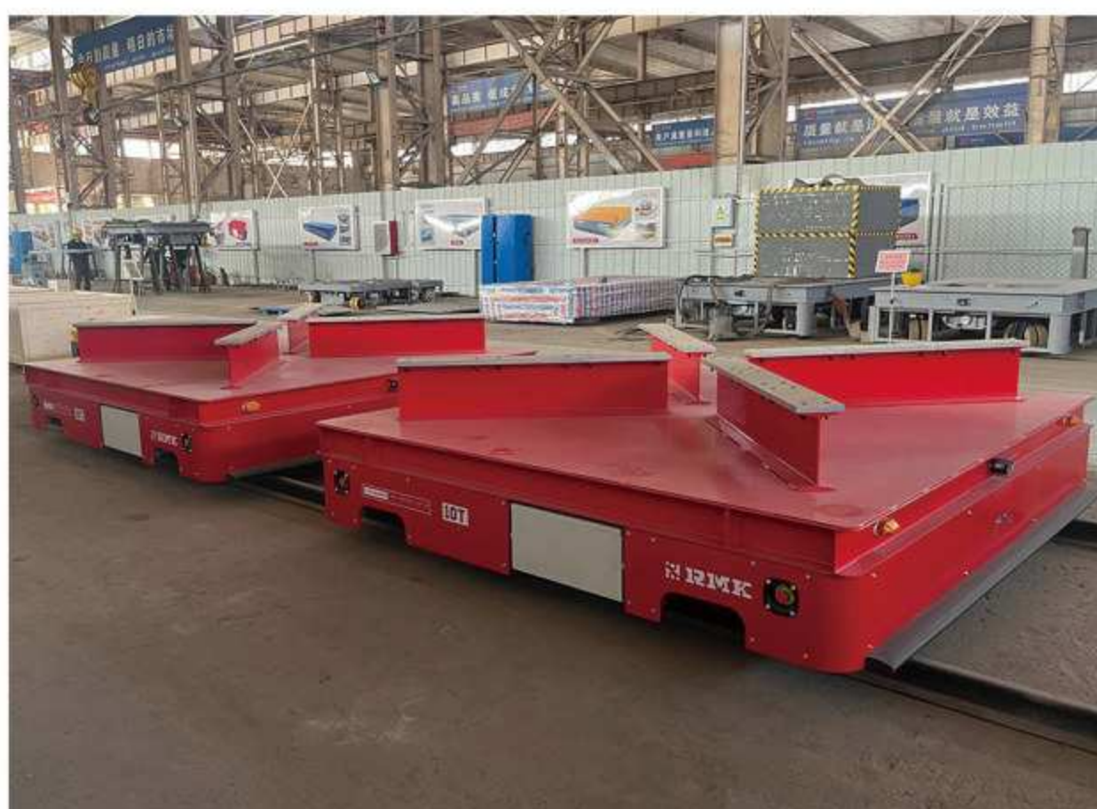
10吨RGV——建筑、高铁桥梁 10 tons RGV - Buildings, High-speed railway bridges
