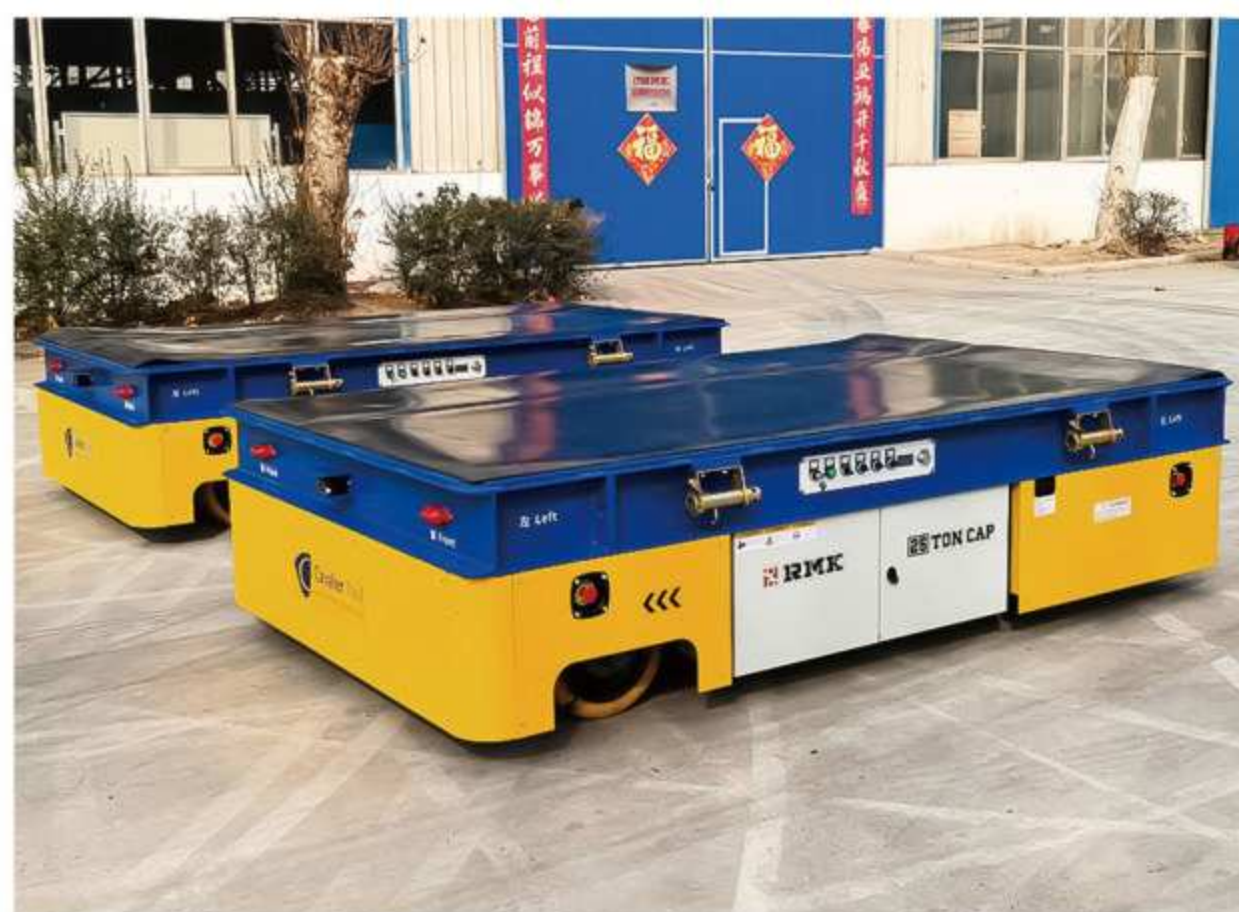
25吨差速无轨车——装备制造 出口加拿大 25 tons trackless transfer cart - Equipment Manufacturing Exported to Canada
