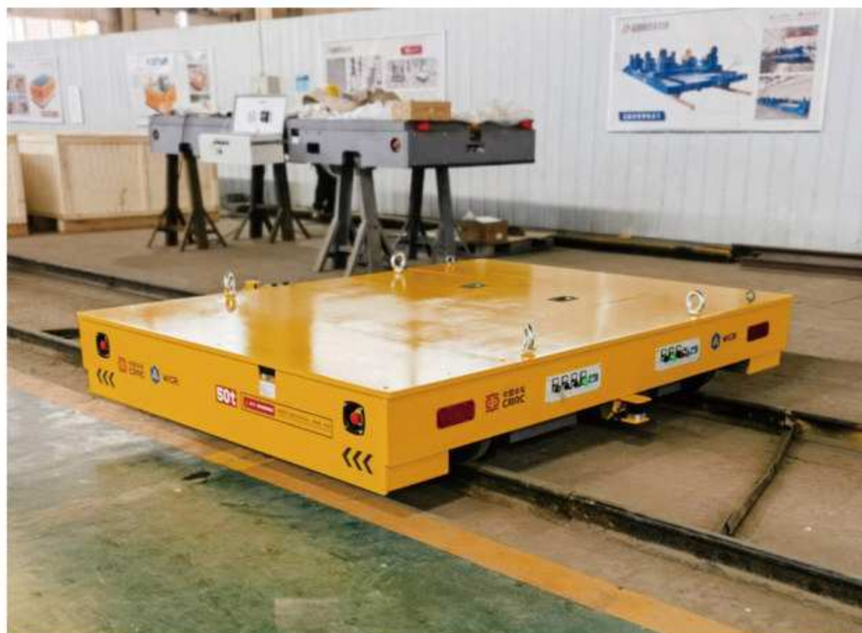
50吨牵引式RGV——车辆制造 50 tons traction RGV - Automotive Manufacturing
