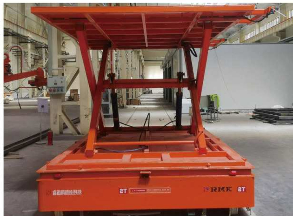
纵横移动自动化轨道车RGV——军工 Vertical and horizontal mobility automated rail car RGV - Military
